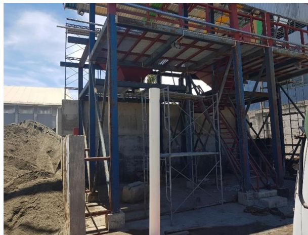
Figure 2-8 Newly installed concrete batch plant at SSS crushing site (~100 m 3 /day capacity); photo by Vilive Anise, 7 November 2020
