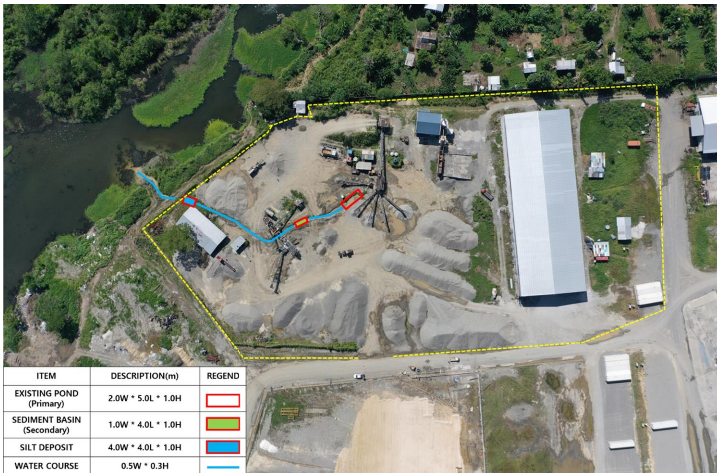
Figure 2-9 Drainage layout (with additional sedimentation basins installed by HEC) at SSS crusher site, Ranadi
