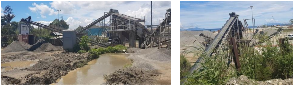
Figure 2-7 Existing crusher plant at SSS: View of whole plant with washer/screening and conveyors (left) and view of conveyor leading to top of washer plant (right); photos courtesy of Vilive Anise (OE), 7 November 2020
