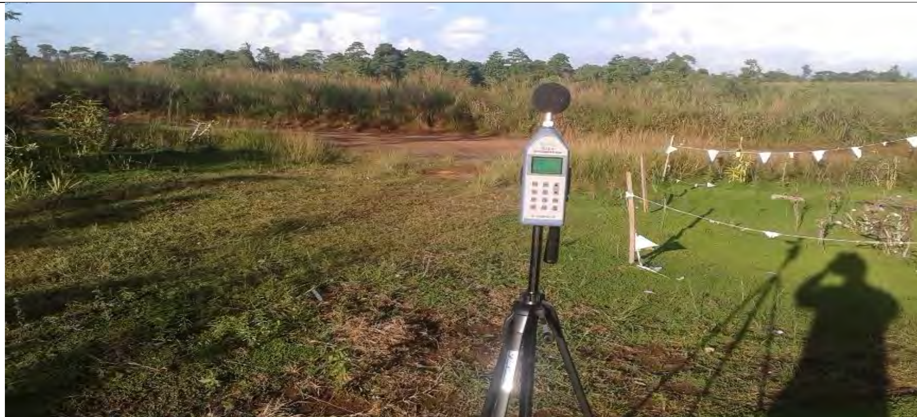
1. Noise monitor set up @Pavu, 5m from the road and 5m from residential building.
