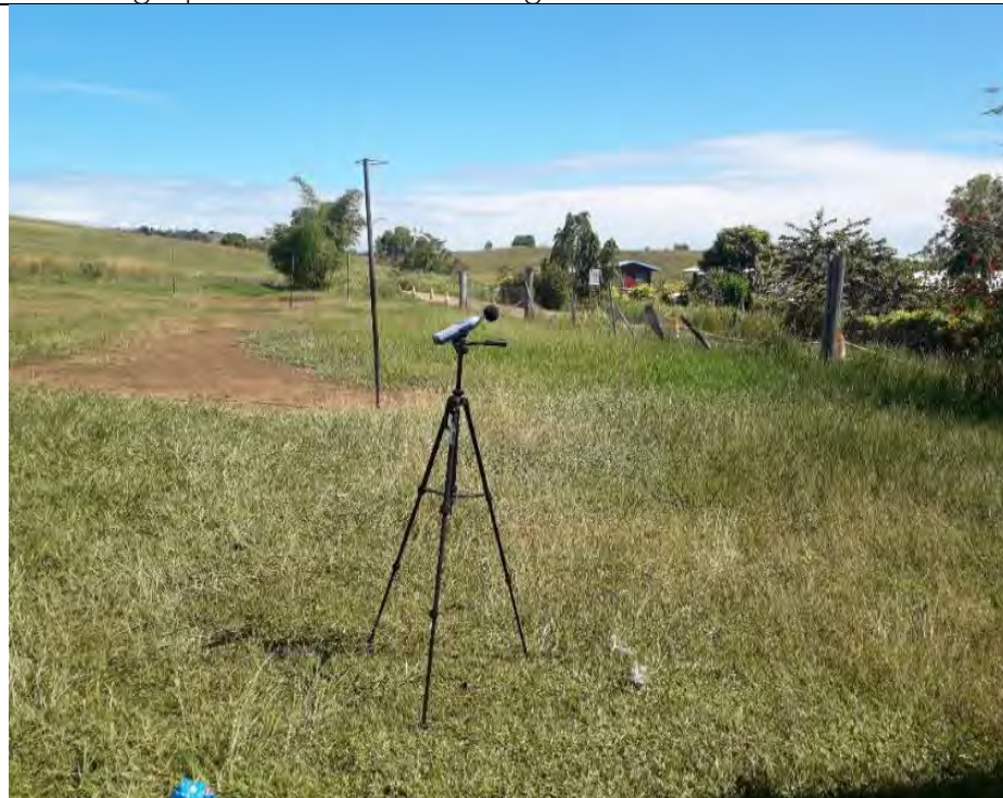
Noise Analyzer set up @ Rate School 5m from the Road (right side) and 10m from school buildings (Ref # 001) 57 L 0622210, 8949443 E
