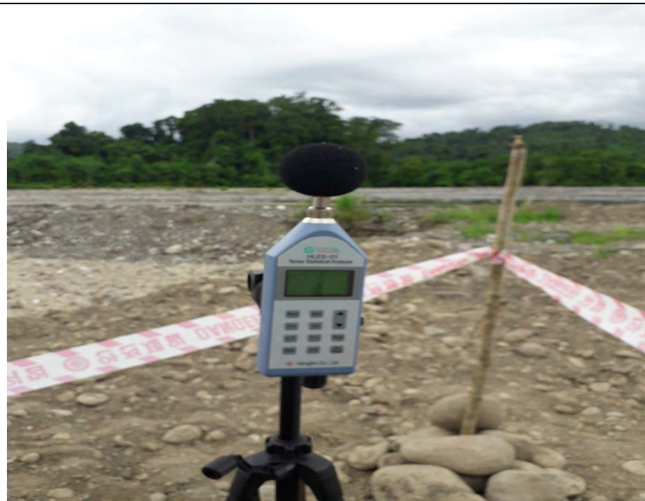
Noise monitoring set up location at Crusher plant 10m from construction site and 20m from the river
